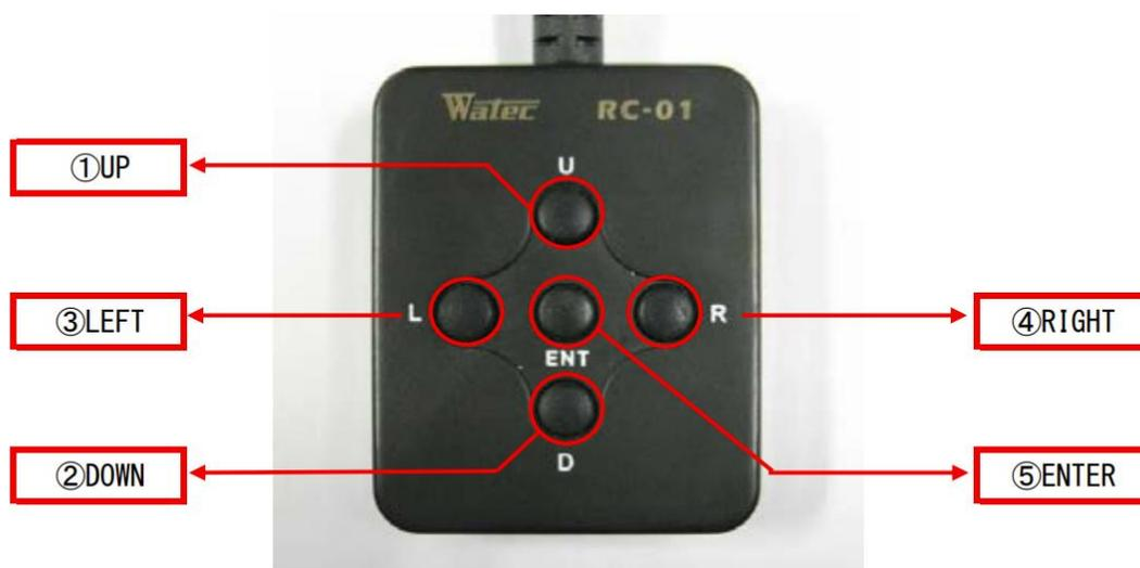
**Figure 1. RC-01 (remote controller)**
